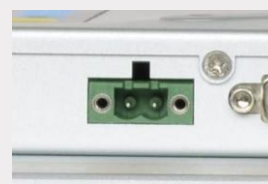
Phoenix terminal using fastening type power connector
